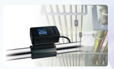
F3CL and F3RO adopts the ultrasonic transit time measurement principle, combined with Gentos' patented flow algorithm technology, it realizes accurate measurement of the fluid flow in the pipe. The product is all-in-one and clip-on structure design, which is simple and convenient to install. Only four steps are needed all along. The installation process requires no contact with fluid media and no need to shut down the flow.
